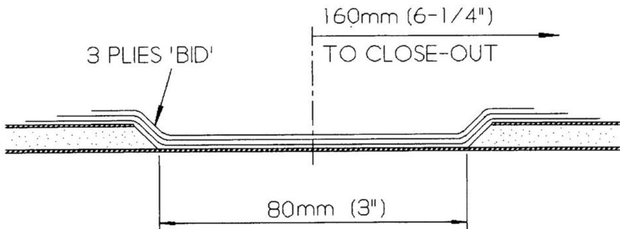
Figure 3 Reinforcement of bottom skin at tailwheel spring front attachment bolt position
