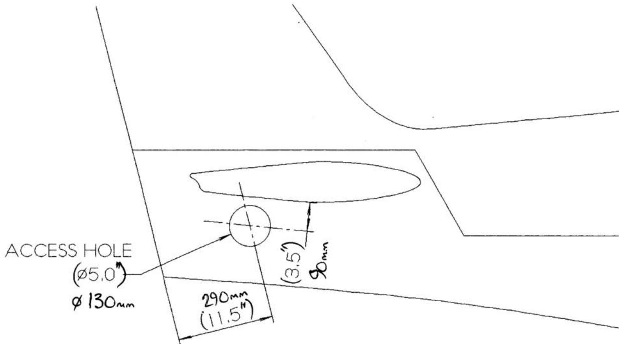
Figure 2 Access hole dimensions and position
