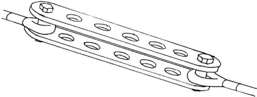
*Figure 12 Cable length adjuster*
