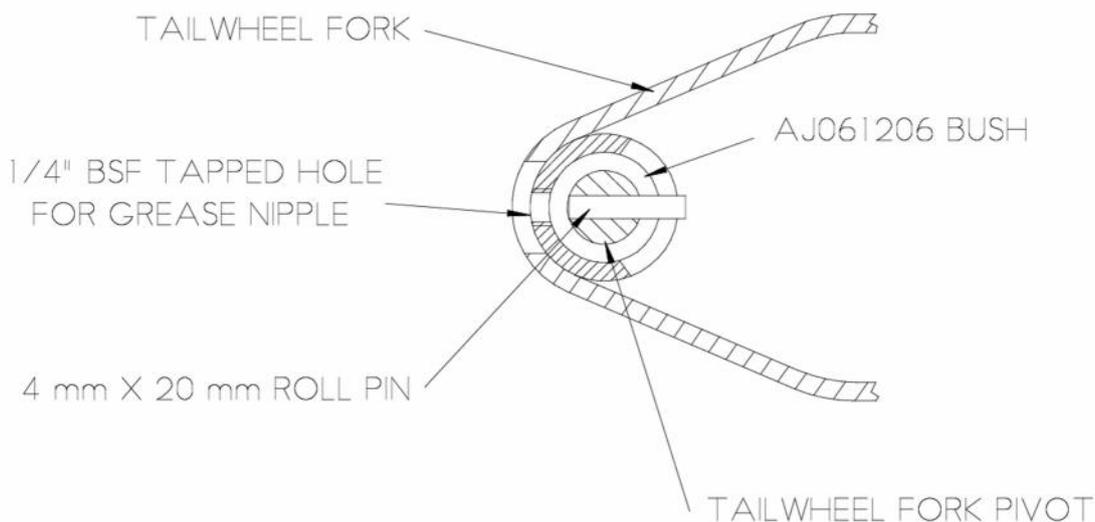
Figure 10 Section showing position of roll pin stop
