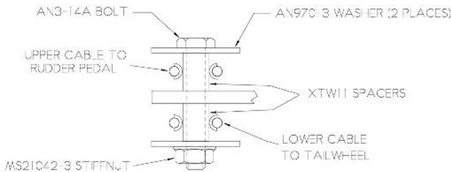
Figure 14 Detail of starboard cable fixing
