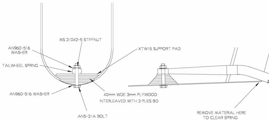
Figure 6 Spring rod forward mountings
