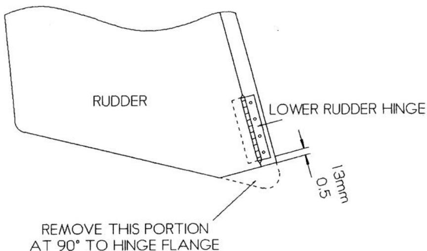
Figure 7 Lower rudder modification for rudder horn
