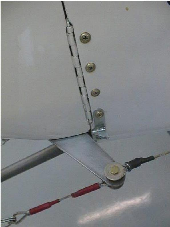
*Figure 15 Tailwheel drive cable*
