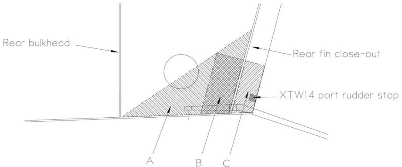
Figure 4 Reinforcement layups
