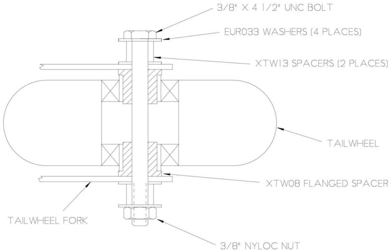
Figure 11 Section through tailwheel axle
