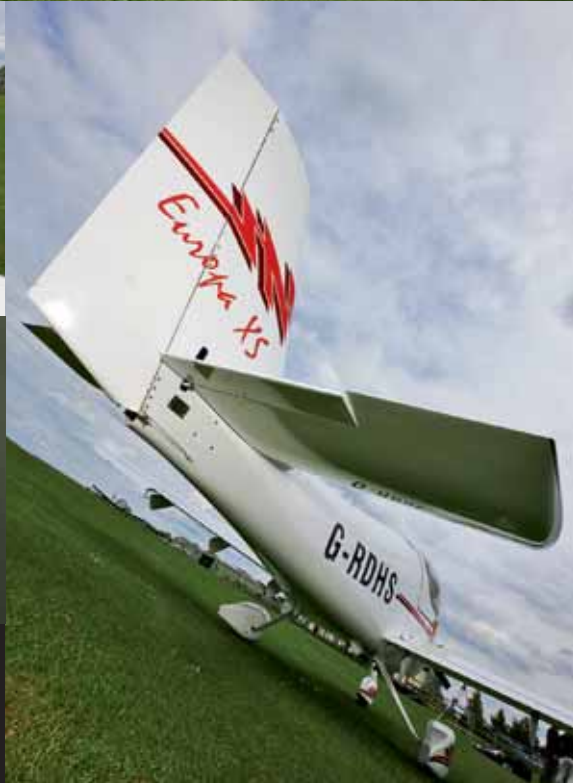
Test aircraft is a Europa XS tri-gear, built by owner Russell Spencer and is a beautifully finished aircraft. Undercarriage knocks 5kt off the cruise speed of the monowheel.
