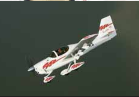
Test aircraft is a Europa XS tri-gear, built by owner Russell Spencer and is a beautifully finished aircraft. Undercarriage knocks 5kt off the cruise speed of the monowheel.
