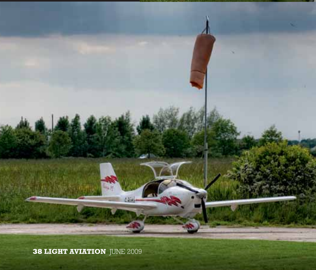
Test aircraft is a Europa XS tri-gear, built by owner Russell Spencer and is a beautifully finished aircraft. Undercarriage knocks 5kt off the cruise speed of the monowheel.
