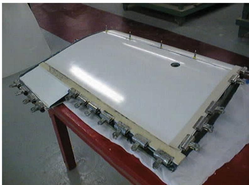
*Fig 7. Holding skin place with spring clips.*
