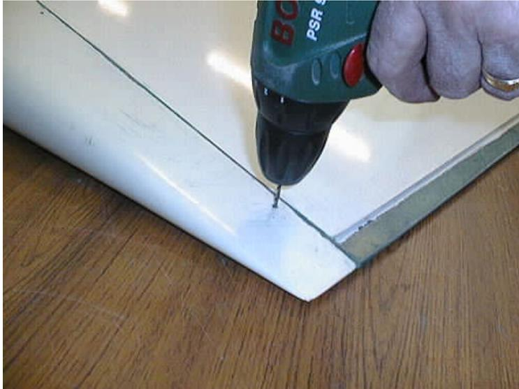
*Fig 12. Drilling venting / drainage hole*
