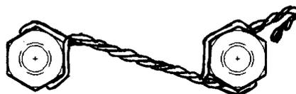
*Fig 5. Typical wire locking detail*
