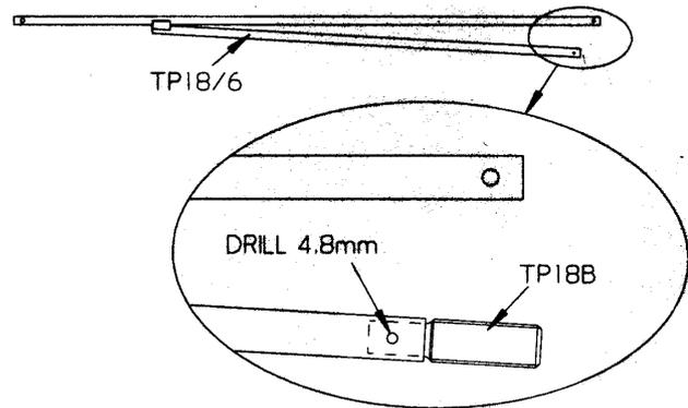
Fig 1. Drilling TP18B
