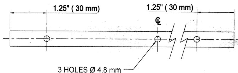
Fig 2. Drilling guide strips.
