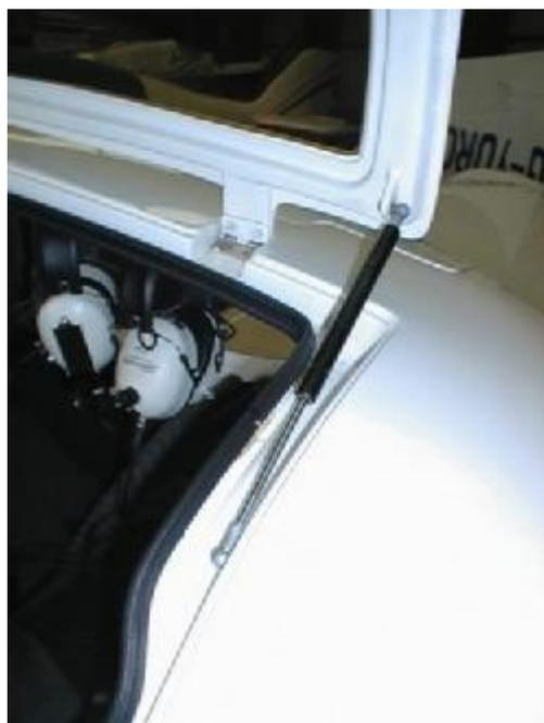
*Fig 1. Original mounting of gas strut.*
