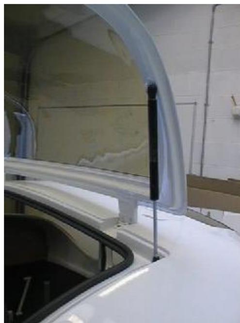
*Fig 2. Revised mounting of gas strut.*
