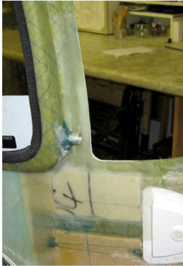
*Fig 10 Finished joint & flange*
