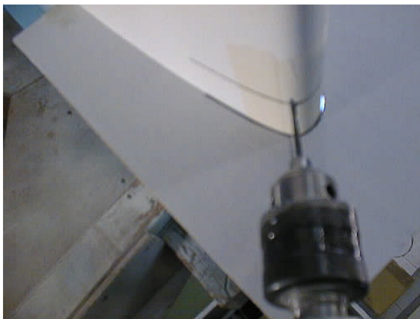
Fig 6. Drilling hole in wing leading edge.
