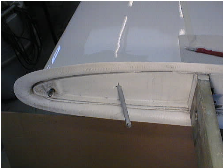
Fig 4. Hole cutter in position.
