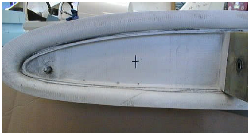
Fig 1. Position of pilot hole.
