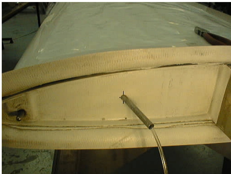
Fig 9. Tubing and cutter at root rib.
