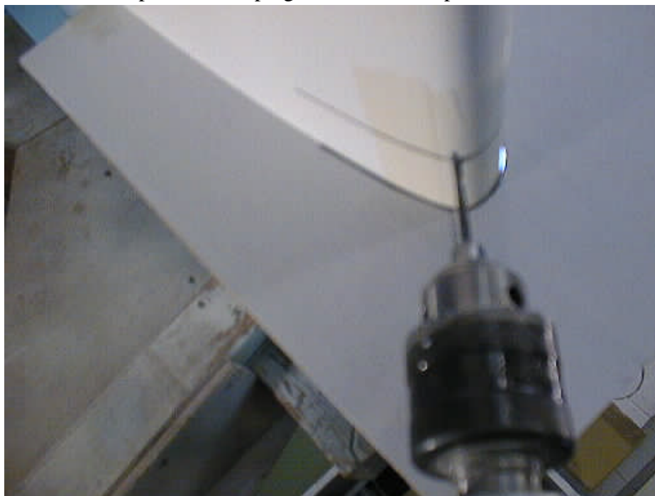
Fig 6. Drilling hole in wing leading edge.
