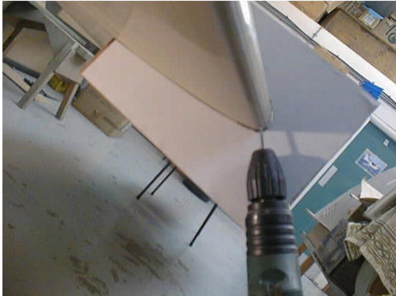
*Fig 7. Drilling pilot hole in leading edge.*
