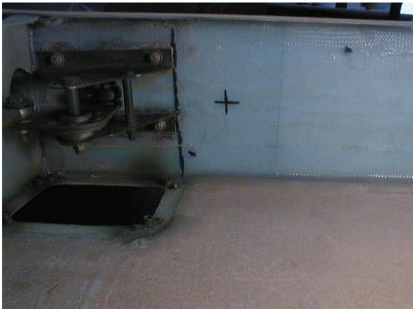
*Fig 1. Marking hole position on spar.*
