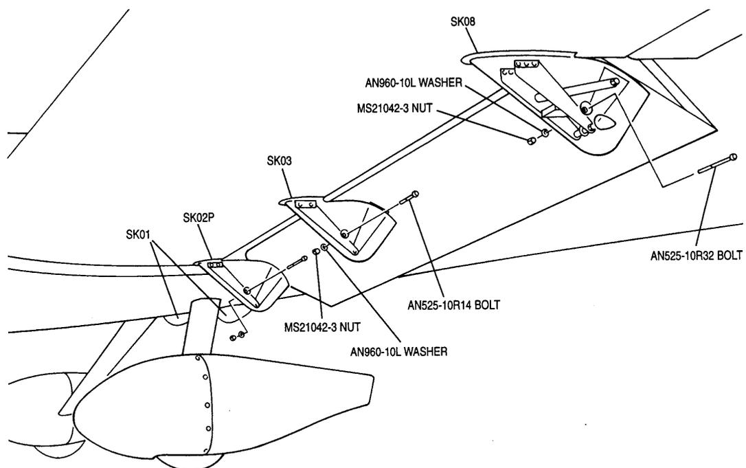
*Fig 1. General arrangement of flap hinge and main gear fairings.*
