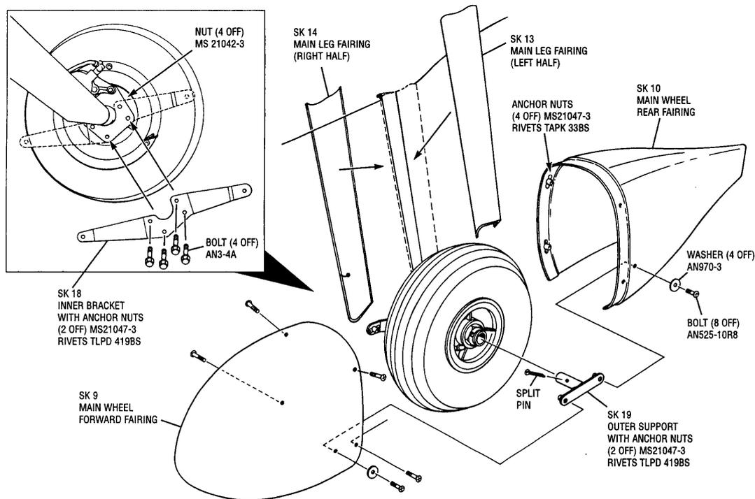
Fig 3. Main Gear Fairings (Port side shown)
