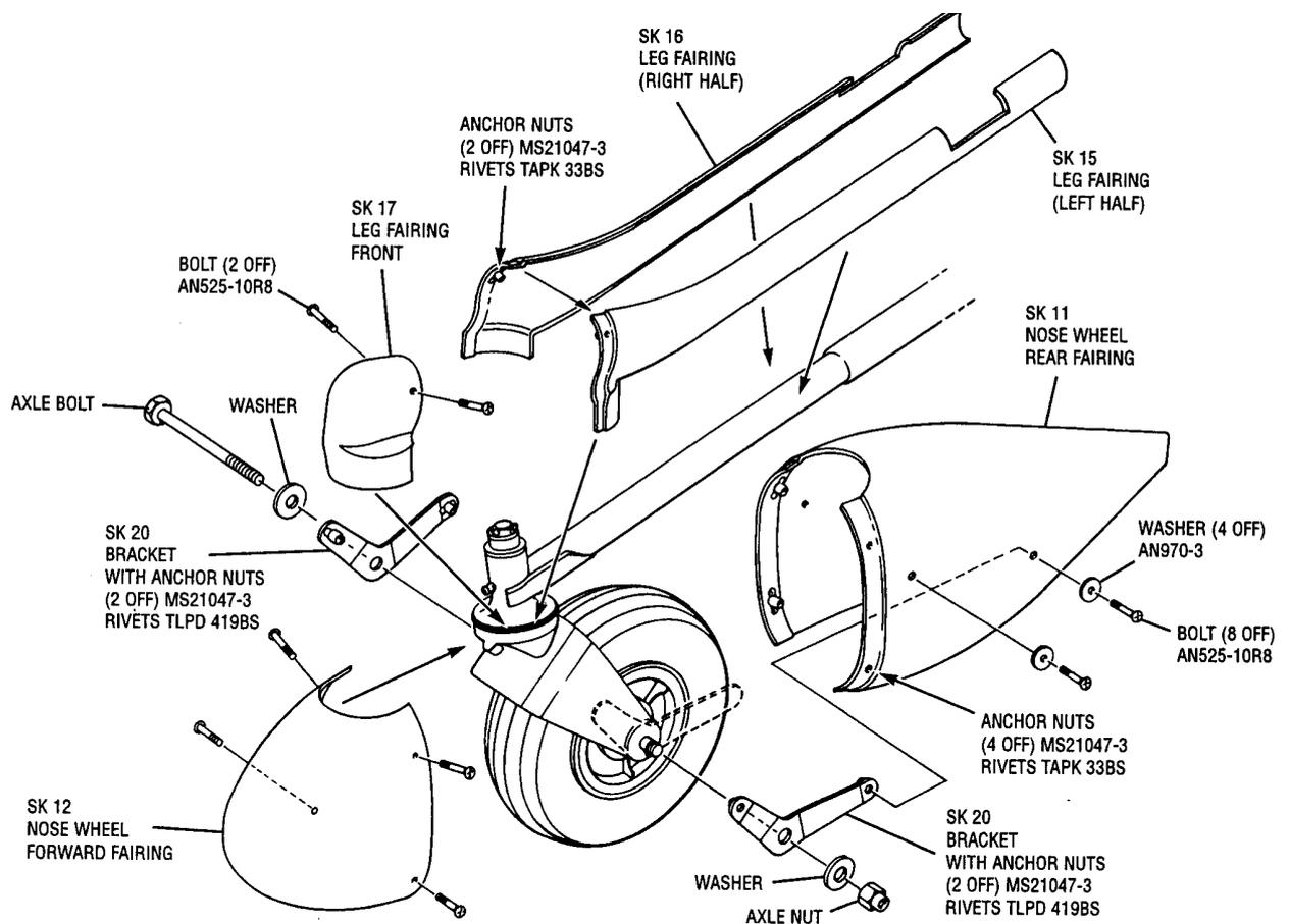
Fig 2. Nose Gear Fairings
