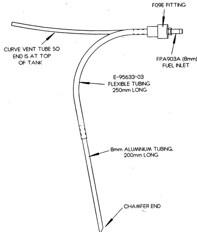
Fig 2. Syphon tube arrangement in vent fitting F09E.
