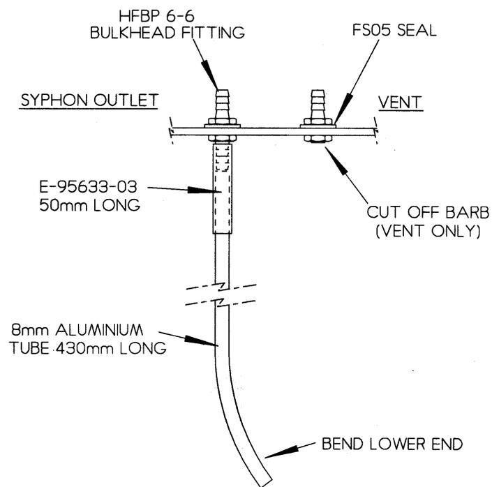
*Fig 4. Fuel outlet and vent arrangement in Long Range tank.*
