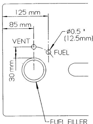
Fig 3. Position of bulkhead fitting holes. View from above.
