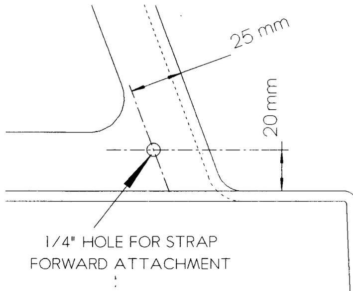
Fig 6. View of starboard side headrest looking outboard.
