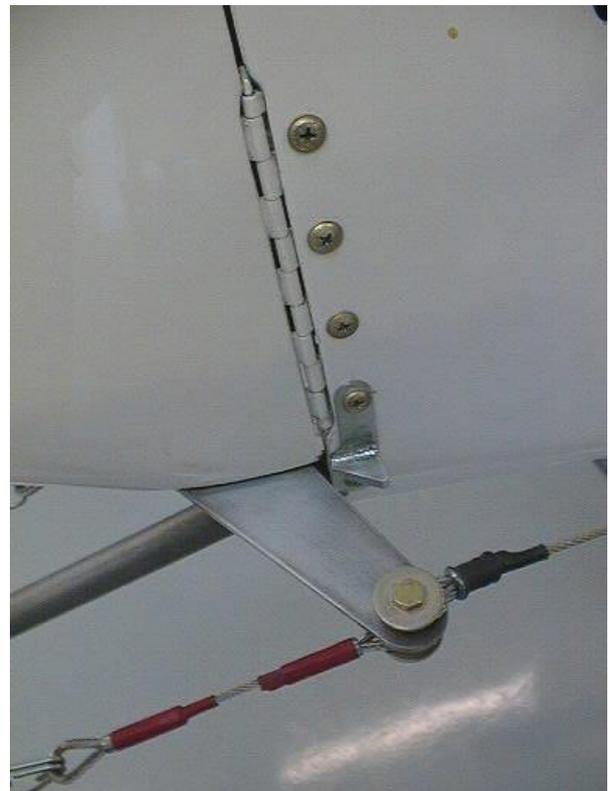
*Fig 14. Tailwheel drive cable.*
