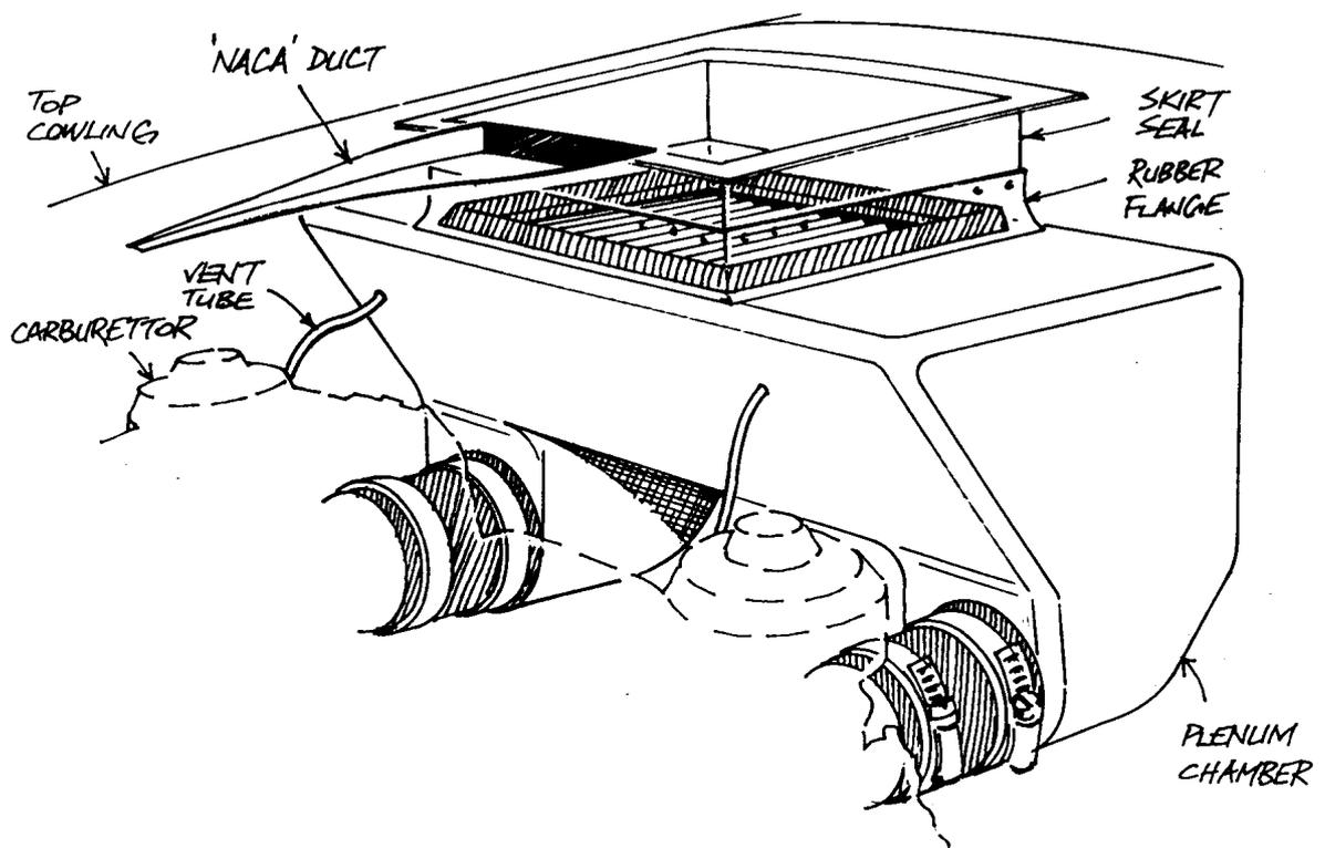
*Fig 1. General arrangement of plenum chamber installation.*
