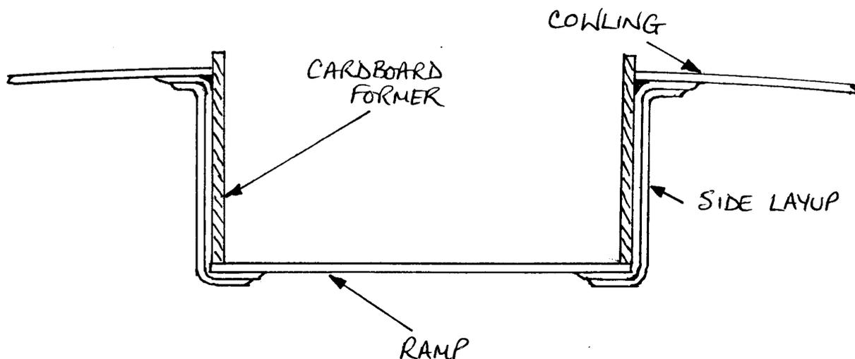
Fig 4. Layup of NACA duct sides.
