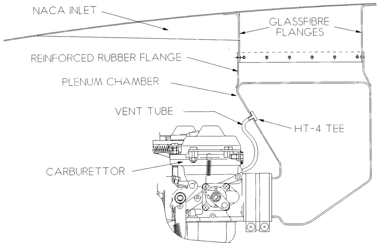
*Fig 5. Sectional view showing NACA duct and skirt seal.*
