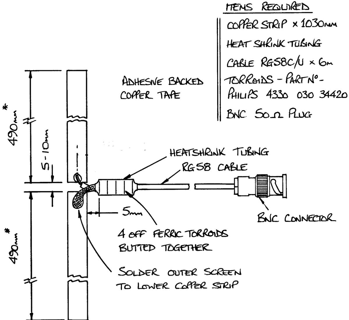
\* NOTE: INITIALLY MAKE COPPER TAPES 515mm LONG EACH AND, CHECKING SIGNAL WITH VSWR METER, SHORTEN TAPES EQUALLY IN 3mm INCREMENTS UNTIL MINIMUM READING COINCIDES WITH 127.5 MHz
