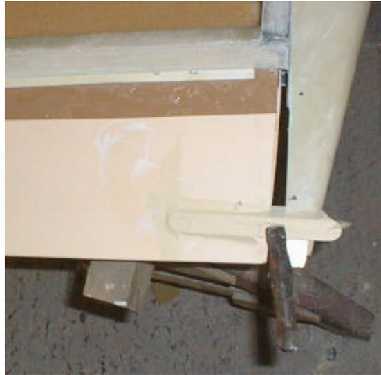
*Fig 29. Aileron clamped in neutral.*
