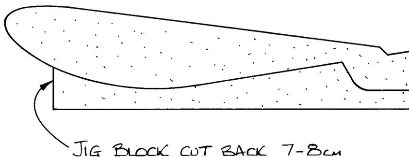
Fig 2. Flap core in jig block.
