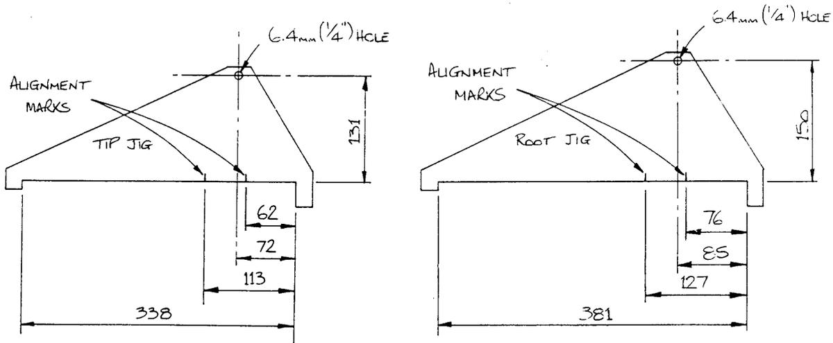
Fig 8. Flap plate positioning jigs (dims in mm).
