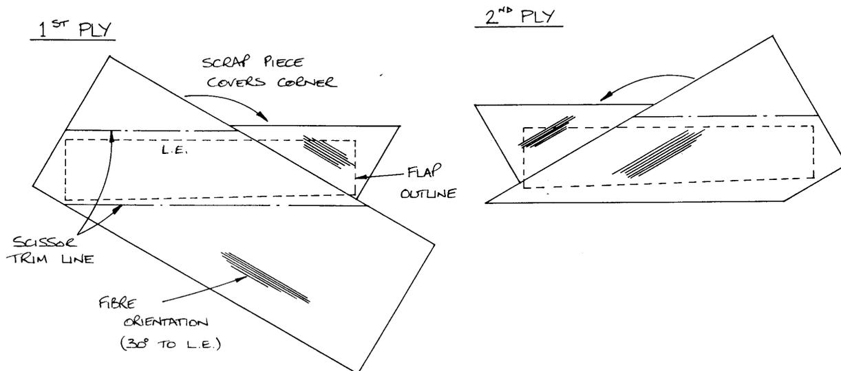
Fig 4. Positioning 'uni' cloth for skin lay-up.
