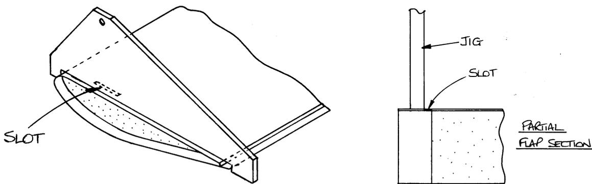
Fig 9. Typical jig position.
