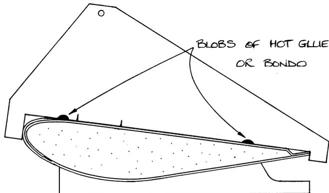
Fig 11. Jig temporarily attached to flap.
