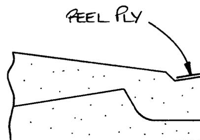
Fig 3. Flap core trailing edge detail.
