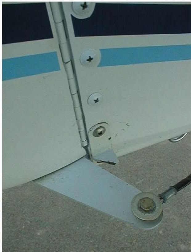
*Fig 5. Photo of starboard rudder stop.*
