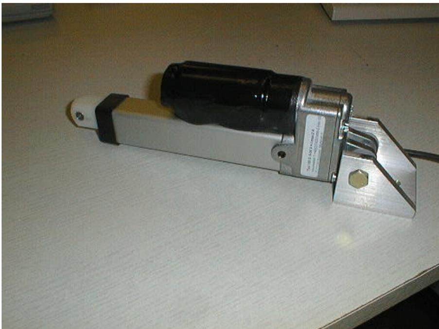
Fig 7. Actuator assembled to mounting bracket.
