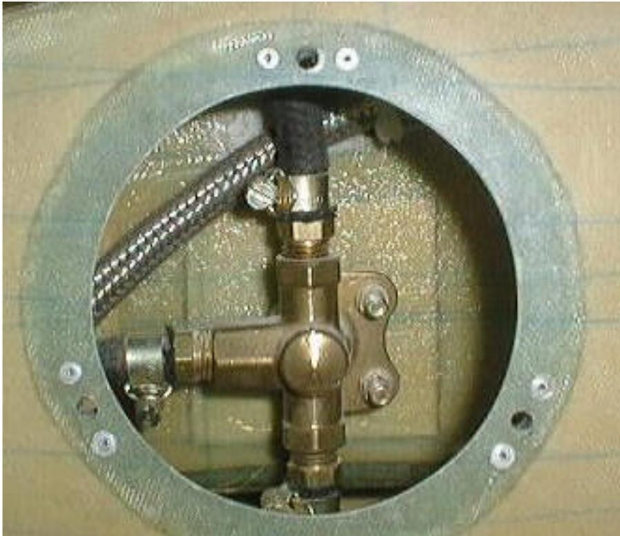
*Fig 1. Fuel selector valve mounting, seen through starboard access hole.*
