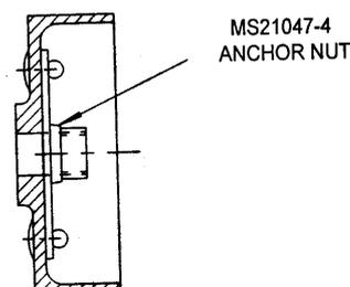
Hold the anchor nut in place by engaging an AN4-10A bolt just finger tight and drill through the lugs, increasing the hole diameter, and the end cap, with a 3.3 mm drill for the rivets. Use two TLPD424BS rivets to fasten each anchor nut then remove the bolt.
