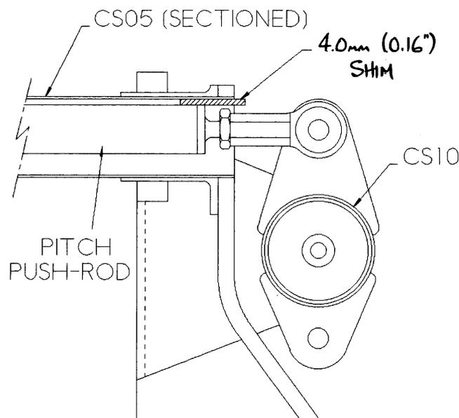
Fig 7. Pitch push-rod to cross-tube assembly.
