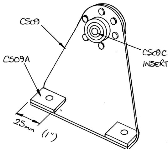
Fig 5. CS09A cuddle plates bonded to CS09 bracket.
