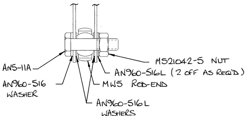
Fig 6. Typical section of rod-end attachment.
