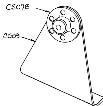
Fig 4. CS09 bracket with CS09B bellcrank assembly.
