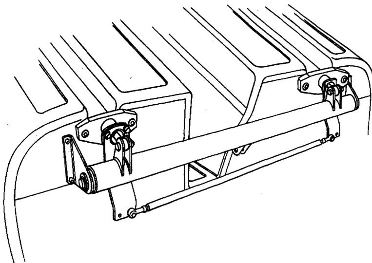
*Fig 1. Installed arrangement of pitch torque tube*
