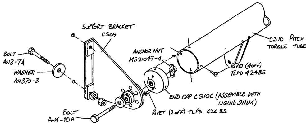
Fig 3. End cap installed in torque tube.
